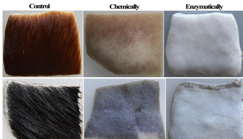
Figure 11: Enzymatic dehairing in the leather industry. (Zhou et al., 2018).
